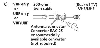
Converter EAC-25 is commercially known as a 300-to-75 ohm antenna adapter.
